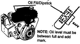
**NOTE:** S.A.E. 5W30 motor oil may be used to make starting easier in areas where the temperature is 20° F. or lower.
